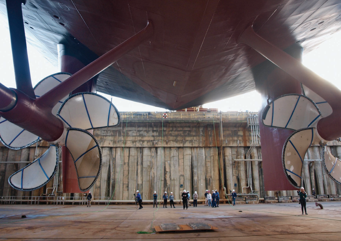
Steelworkers, sailors, and others involved in the building of Kennedy check below the hull before the dry dock is flooded and the ship is launched.
