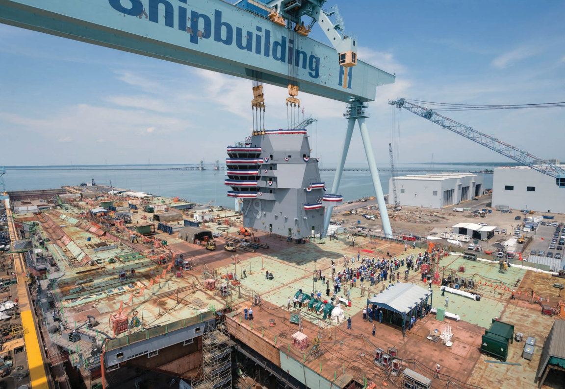
Big Blue prepares to set carrier Kennedy 's island on the ship deck, marking another major milestone in the vessel's construction.
